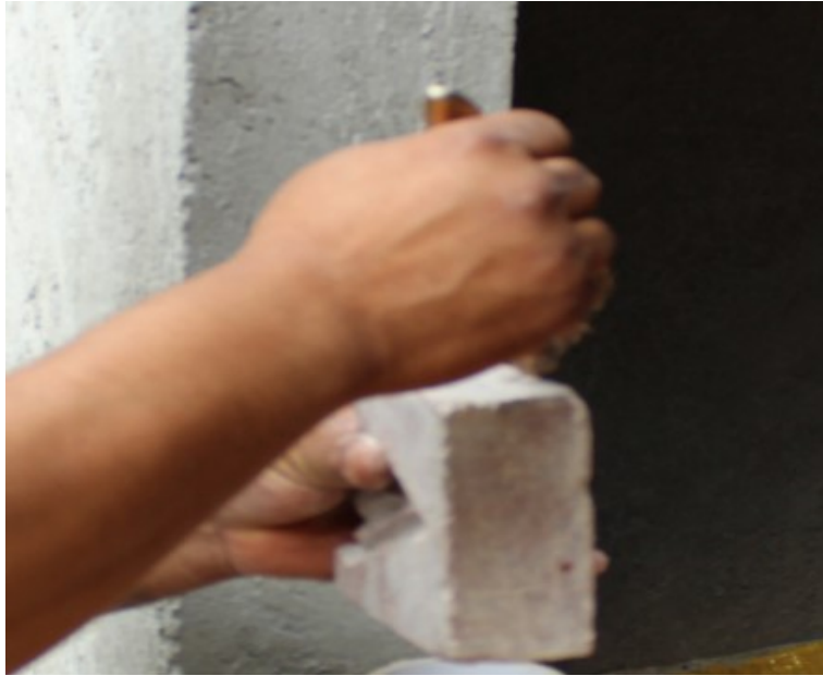
Fig. 5. The materials were applied on bricks, in order to determine waterproofing
