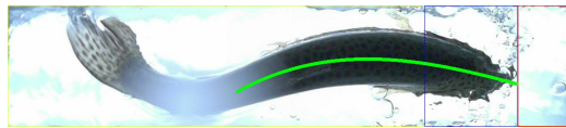
Figure 11: A sample when the fish body could not be detected completely due to high contrast.
