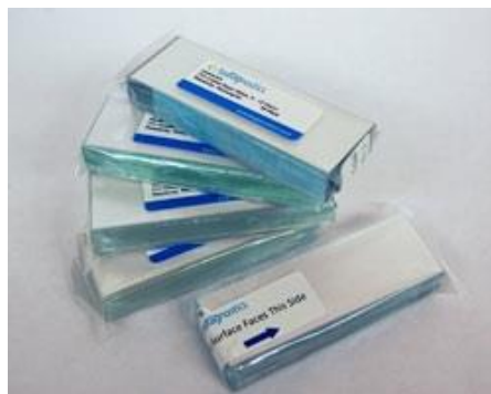
Figura 7. Sustrato de ITO Cytodiagnosics ( 8\text{-}12\Omega/\text{square} ).
