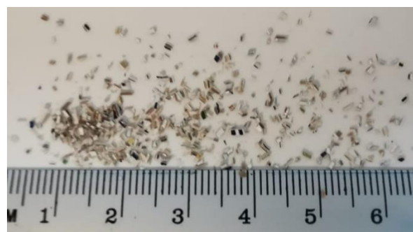
Figure 2. Tetra Pak particles cut with scissors (Authors' elaboration).
