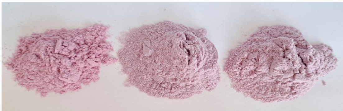
Figure 2. PPCb encapsulated by freeze-drying. a) Using M as wall material; b) Using GA as wall material; c) Using M-GA in a 1:1 ratio (M-GA) as a wall material.
