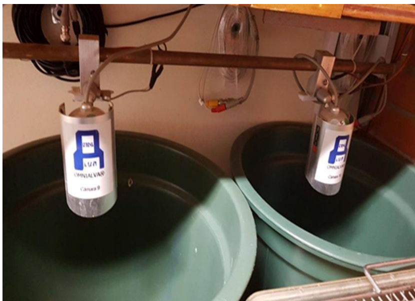
Figure 7.2 Automatic lap counter for turning test
