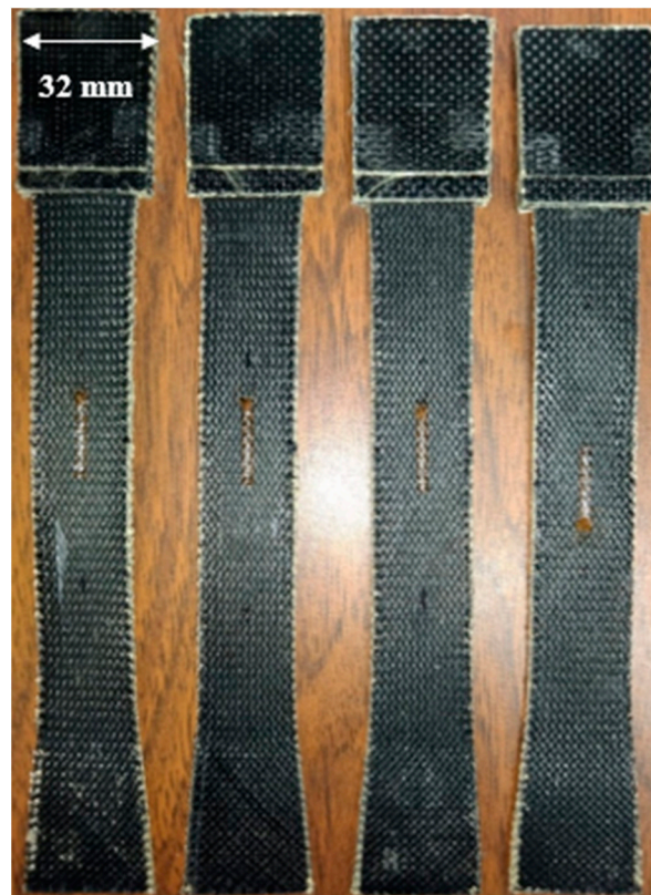
Figure 16. Condition of coupons after the tensile tests at [+45^\circ, -45^\circ]_s .
