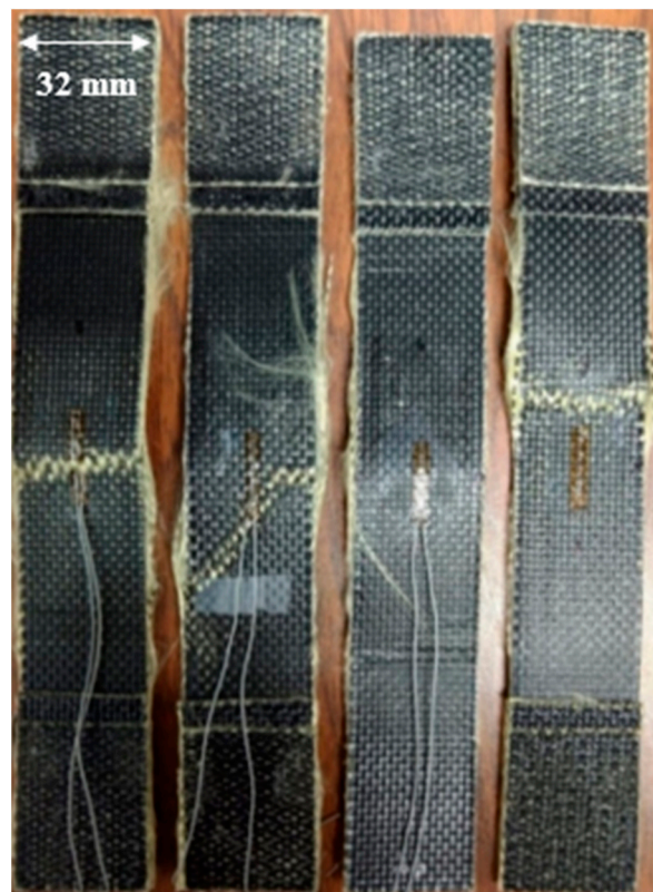
Figure 13. Condition of coupons after the tensile tests at 90^\circ .
