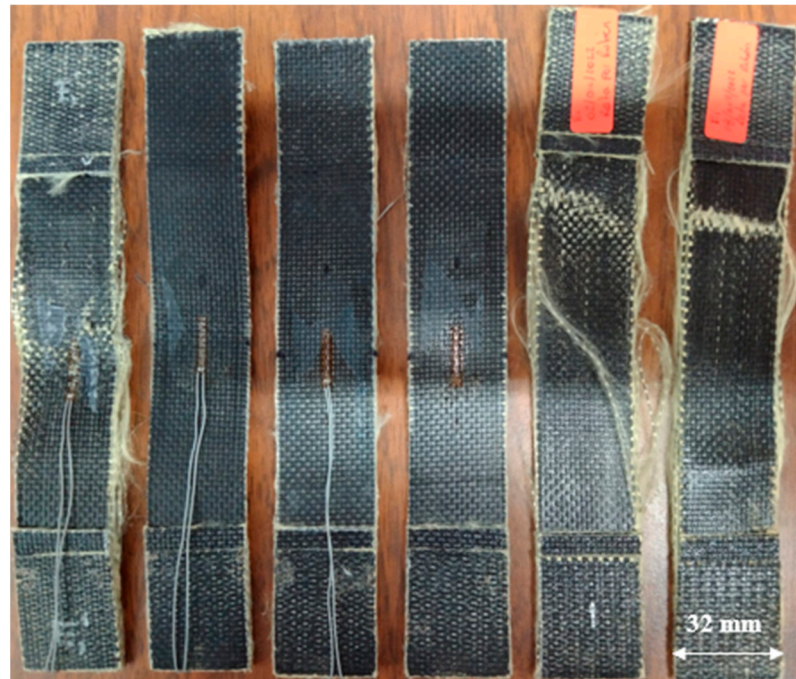
Figure 11. Condition of coupons after the tensile test at 0°.
